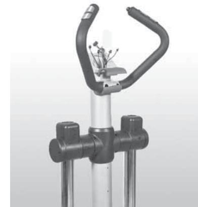
Thread the handgrip pulse cables inside the front tube and pull them out through the top end of the tube. Attach the stationary handlebar with two screws. **NOTE!** Beware not to damage the cables!
