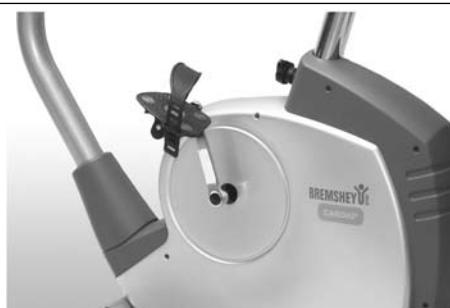
Screw the pedals into the threads of the crank arms. Screw the left pedal (marked L for left-hand thread) into the left crank arms. Use the wrench and rotate it counterclockwise. Screw the right pedal (marked R for right-hand thread) tightly clockwise into the right crank arm. Now attach the pedal straps to the pedals.
