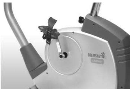
Screw the pedals into the crank arms. Screw the left pedal (marked L for left-hand thread) into the left crank arm. Use the wrench and rotate it counterclockwise. Then screw the right pedal (marked R for right-hand thread) tightly clockwise into the right crank arm. Now attach the pedal straps to the pedals and adjust as desired.
