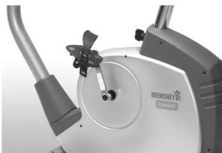
Screw the pedals into the crank arms. Screw the left pedal (marked L for left-hand thread) into the left crank arm. Use the wrench and rotate it counterclockwise. Then screw the right pedal (marked R for right-hand thread) tightly clockwise into the right crank arm. Now attach the pedal straps to the pedals and adjust as desired.
